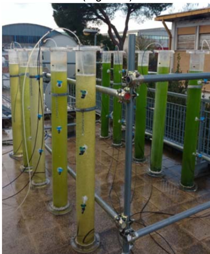
Figure 1: Pilot plant located inside Bio-P s.r.l.; in this particular test, five reactors were inoculated with Scenedesmus obliquus (right) and five with Graesiella emersonii (left).
