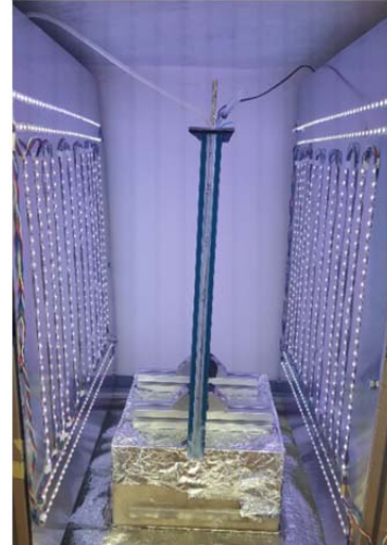
Figure 2: Picture of “quasi-isoactinic” reactor set up. LED panels are positioned at a certain distance from the reactor in order to provide a homogeneous light distribution on reactor's walls.
