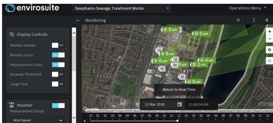
Figure 1: Monitoring H 2 S in real time and 'arc of influence' indicating area for investigation
