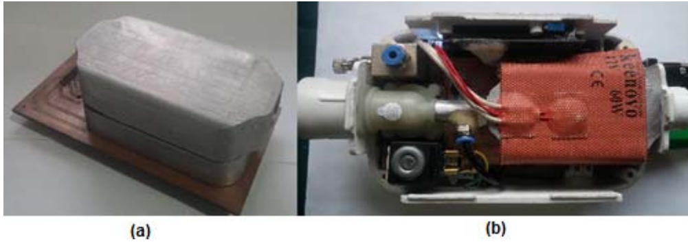
Figure 3: (a) multisensory chamber, (b) top view SOE-I device
