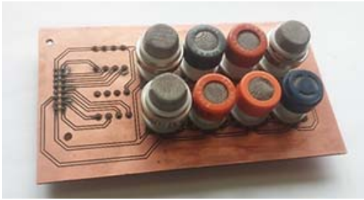
Figure 1: (a) SOE-I sensor array
