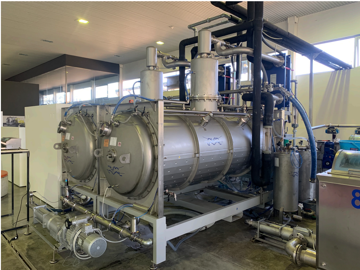
High vacuum malaxers in a industrial olive oil mill.
