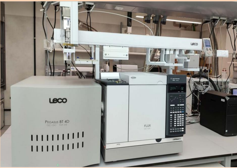
Figure 3. Two-dimensional gas chromatography in combination with mass spectrometry to create aroma maps for the wines.
